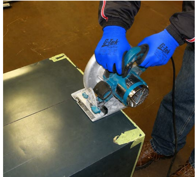
Figure 5. Cutting along marked line
