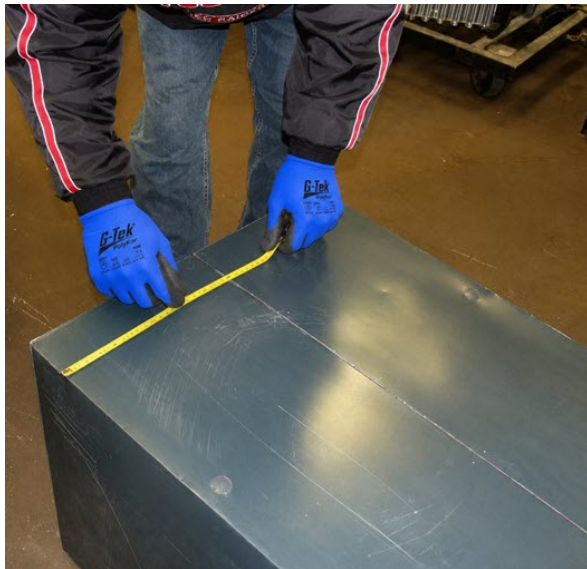
Figure 4. Marking dimensions on back of the cabinet
